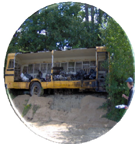
Leaky outdoor parts storage areas like this school bus (above) should be retrofitted to limit contact with precipitation.
