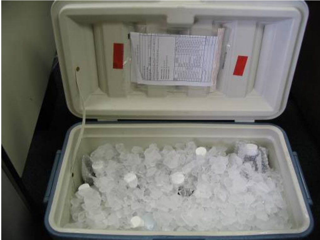
Stormwater samples packed for delivery to the lab, note the chain of custody forms attached to the lid.
