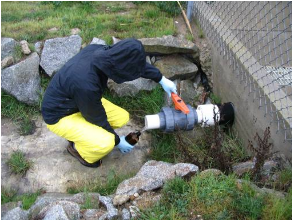
Stormwater discharges to the slot drain and is conveyed offsite through a valved pipe.
