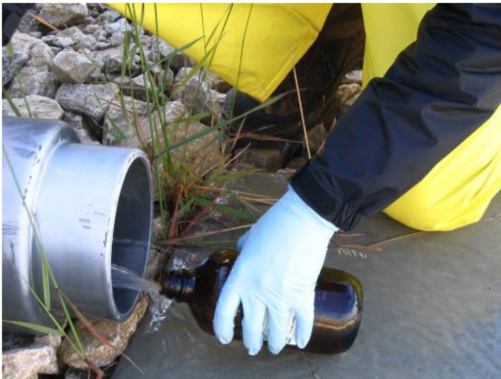
A stormwater grab sample is collected directly into the sample container.
